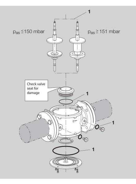
Check the valve seat: if the valve seat is damaged, dismantle the unit and send it to the manufacturer.
