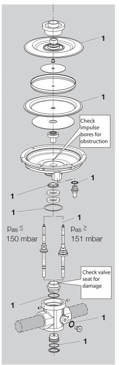
Check the valve seat: if the valve seat is damaged, dismantle the unit and send it to the manufacturer.
